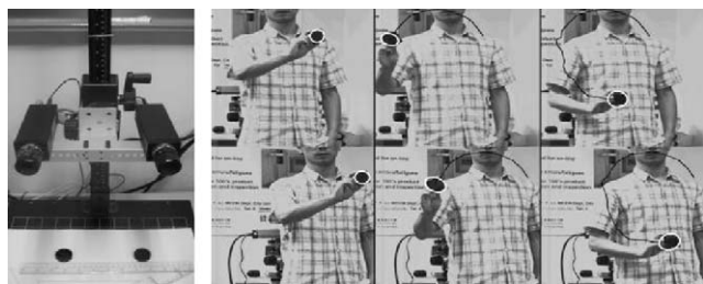
Fig. 5. The vision system setup and snaps of the stereo trajectory tracking.
