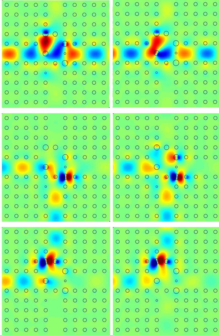
Fig. 3. Left: Electric field patterns for a given incident wave in the left-horizontal waveguide at the three target frequencies. From top to bottom,  $\omega a/2\pi c = 0.36, 0.37, 0.38$ . Right: Electric field patterns of three leaky modes. From top to bottom,  $\omega a/2\pi c = 0.35972 - 0.00402i, 0.37017 - 0.00078i, 0.38044 - 0.00109i$
