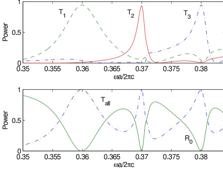
Fig. 2. (a) Normalized transmitted powers in the three output waveguides. (b) Total normalized transmitted power in the output waveguides and the reflected power in the input waveguide.
