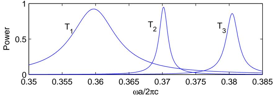
Fig. 4. Transmitted powers to three output waveguides based on the resonant modes and the temporal coupled mode theory.
