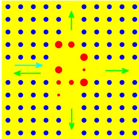
Fig. 1. Three-frequency wavelength demultiplexer in a square-lattice photonic crystal.
