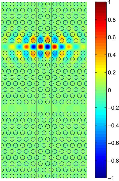
Fig. 9. The magnetic field pattern of a resonant mode of the leaky mode-gap cavity.
