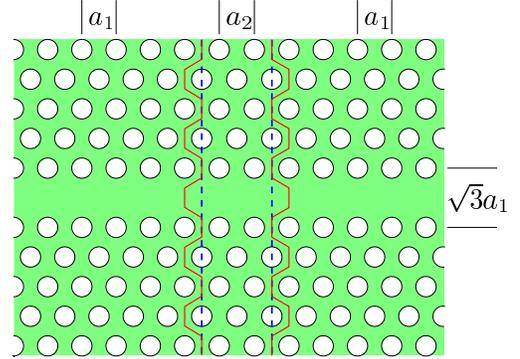
Fig. 6. A mode-gap cavity constructed by connecting a small segment (length  $2a_2$ ) of PhCW2 with two semi-infinite segments of PhCW1.
