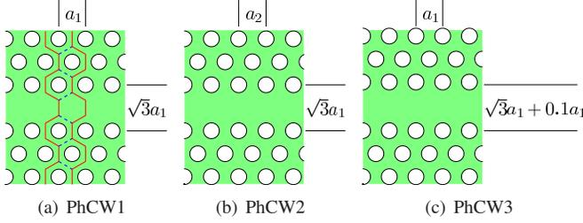
Fig. 1. Three different PhC waveguides. PhCW1: standard line-defect waveguide; PhCW2: horizontally stretched waveguide; PhCW3: waveguide with increased core width. The  $x$  and  $y$  axes point to the horizontal and vertical directions, respectively.
