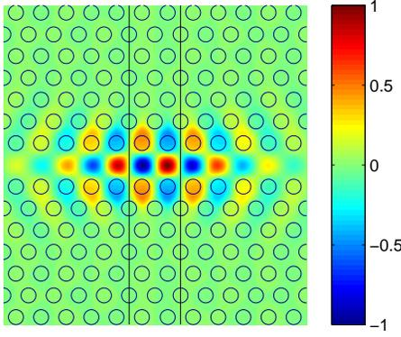
Fig. 7. The magnetic field pattern of a resonant mode of a mode-gap cavity.
