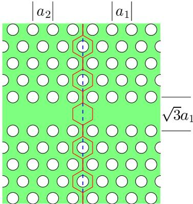
Fig. 4. Waveguide discontinuity in a PhC heterostructure. The left and right half planes are the PhC waveguides shown in Fig. 1(b) and Fig. 1(a), respectively.
