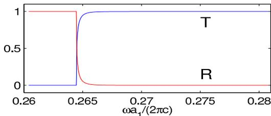
Fig. 5. Transmission and reflection spectra of a waveguide discontinuity in a PhC heterostructure.
