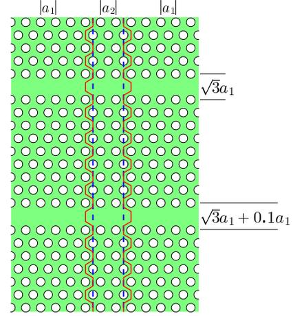
Fig. 8. A mode-gap cavity coupled with the third waveguide shown in Fig. 1(c).
