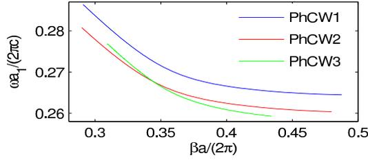
Fig. 3. Calculated dispersion curves for waveguides PhCW1, PhCW2 and PhCW3. The horizontal axis is  $\beta a/(2\pi)$  where  $a = a_1$  for PhCW1 and PhCW3, and  $a = a_2$  for PhCW2.
