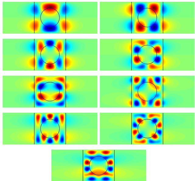
Fig. 5. Magnetic field patterns of the nine standing waves on a slab ( $\varepsilon_1 = 11.6$ ) with an array of air-holes.
