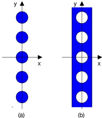
Fig. 1. Two periodic waveguides: (a) a periodic array of dielectric cylinders; (b) a dielectric slab with a periodic array of air-holes.
