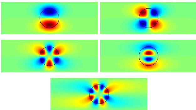
Fig. 3. Electric field patterns of the five standing waves on a periodic array of cylinders with  $r = 0.30a$  and  $\varepsilon_1 = 11.6$ . The frequencies are  $\omega a / 2\pi c = 0.4112, 0.5897, 0.7842, 0.8590,$  and  $0.9766$ .
