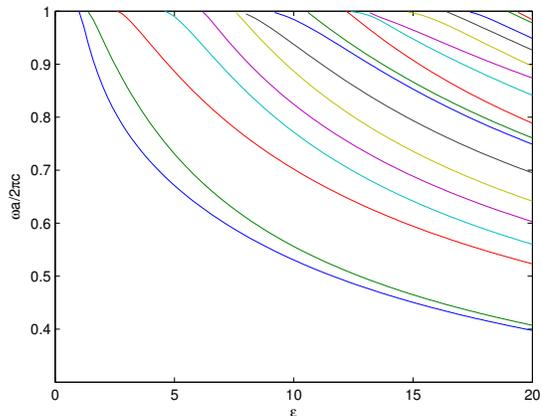
Fig. 4. Frequencies of standing waves on a dielectric slab with an array of air-holes of radius  $r = 0.3a$ .
