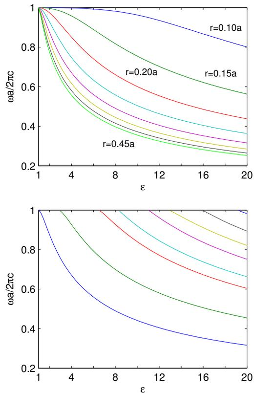
Fig. 2. Top: Standing wave with the smallest frequency on periodic arrays of circular cylinders with radius  $r$  and dielectric constant  $\varepsilon_1$ . Bottom: Frequencies of all standing waves on an array of circular cylinders with radius  $r = 0.3a$ .
