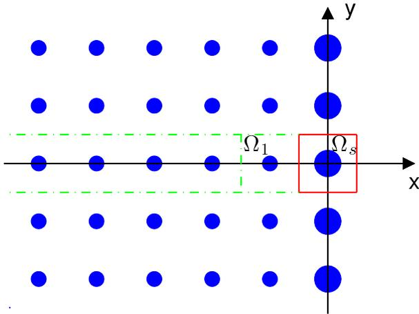
**Fig. 1.** A 2D semi-infinite PhC structure consisting of dielectric rods on a square lattice. The rods are parallel to the  $z$  axis and surrounded by air. The array along the  $y$  axis corresponds to the surface of the structure.
