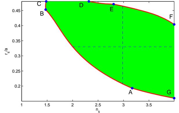
**Fig. 2.** Existence domain in the  $n_s r_s$  plane for a BIC propagating along the surface of the 2D PhC structure shown in Fig. 1, where  $n_s$  and  $r_s$  are the refractive index and radius of the surface rods.
