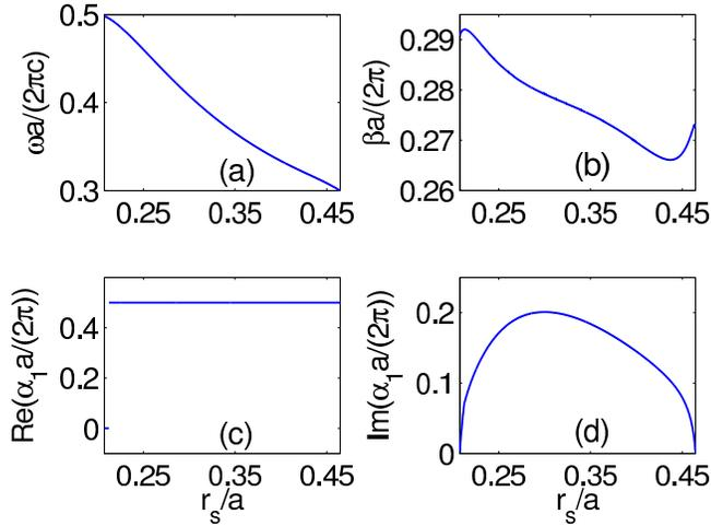
**Fig. 4.** (a) and (b): Frequency and wavenumber of the BIC as functions of  $r_s$  for  $\epsilon_s = 8.9$ . (c) and (d): Real and imaginary parts of  $\alpha_1$ , corresponding to the Bloch mode in the bulk PhC with the slowest decay rate in  $x$ .
