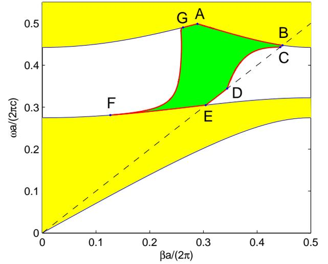
**Fig. 6.** Projected band structure (yellow regions) of the bulk PhC with rod radius  $r_1 = 0.2a$  and dielectric constant  $\epsilon_1 = 8.9$ , and frequency-wavenumber domain (green region) of the BICs for  $r_s$  and  $\epsilon_s$  shown in Fig. 2.
