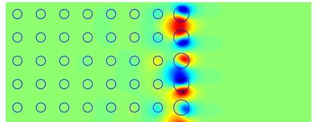
**Fig. 3.** Electric field pattern (real part of  $u$ ) of a BIC for the PhC structure shown in Fig. 1 with  $r_s = 0.33a$  and  $\epsilon_s = 8.9$ .
