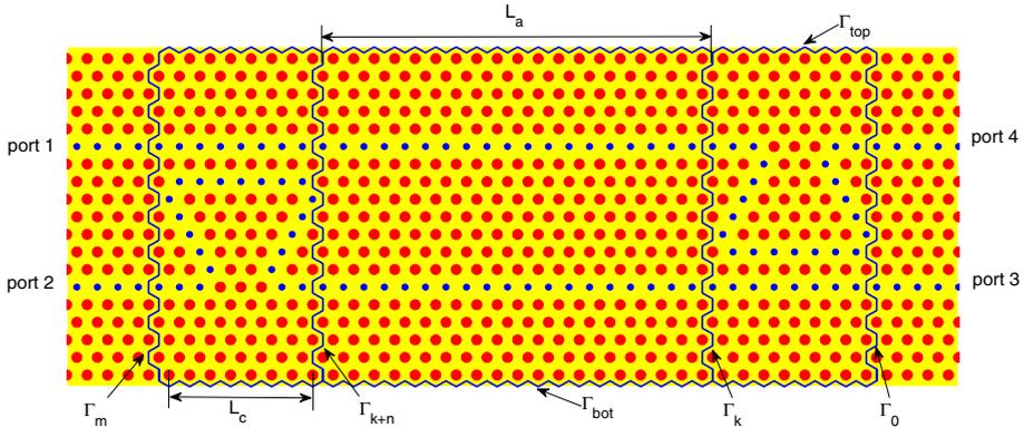
**Fig. 2** Mach-Zehnder interferometer proposed in Fujisawa and Koshiba (2006) based on photonic crystal waveguides in a triangular lattice
