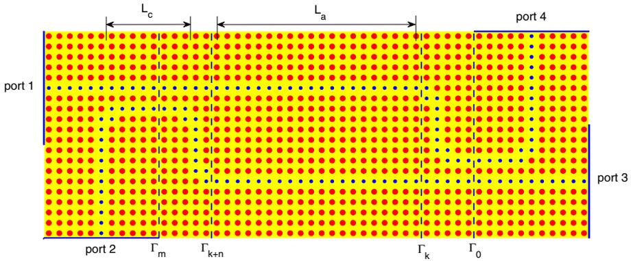
**Fig. 4** Mach-Zehnder interferometer proposed in Fujisawa and Koshiba (2006) based on photonic crystal waveguides in a square lattice
