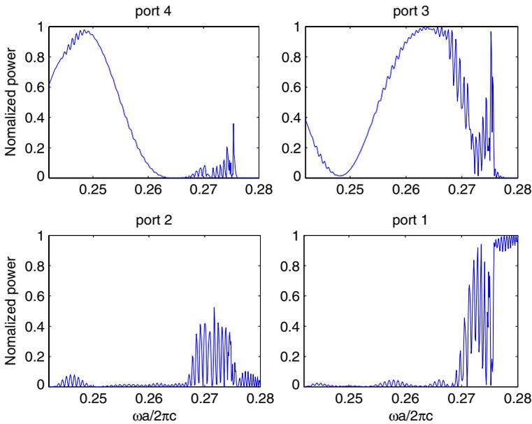
**Fig. 5** Normalized output power in the four ports as a function of  $\omega a / (2\pi c)$  for the Mach-Zehnder interferometer shown in Fig. 4
