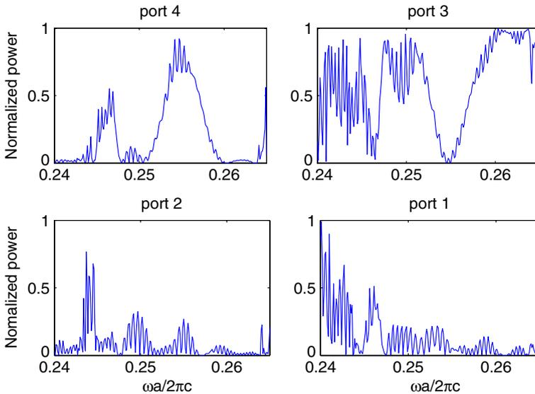
**Fig. 3** Normalized output power in the four ports as functions of  $\omega a / (2\pi c)$  for the Mach-Zehnder interferometer shown in Fig. 2
