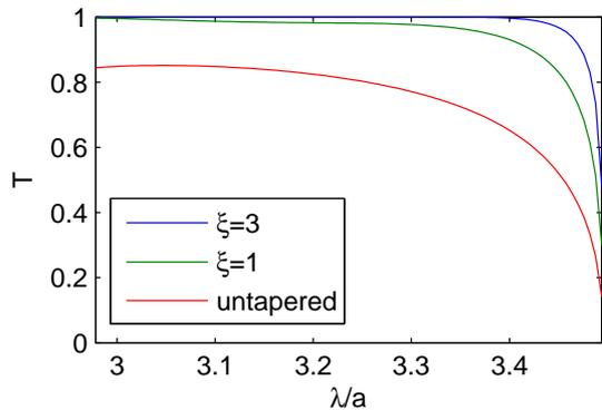
Fig. 4. Transmittance of the tapered and untapered photonic crystal waveguides shown in Fig. 3.
