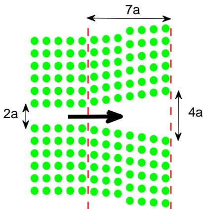
Fig. 3. A PhC waveguide and free space connected by a seven-layer taper.
