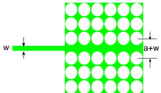
Fig. 1. Direct connection between a PhC waveguide with a slab waveguide.
