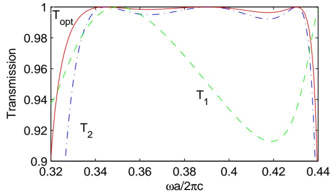
Figure 4: Transmission spectra of three different  $90^\circ$  photonic crystal waveguide bends.  $T_1$ ,  $T_2$  and  $T_{opt}$  correspond to the bends in [2], [8] and in Fig. 3, respectively.
