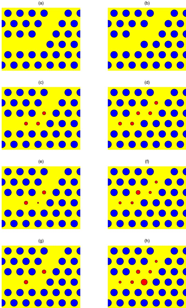
Figure 1: Waveguide bends in a 2D photonic crystal with a triangular lattice of air-holes. (a) The standard  $60^\circ$  bend; (b) The longer bend; (c,d) Improved bends by Chutinan *et al.* [7]; (e-h) Optimized  $60^\circ$  waveguide bends.
