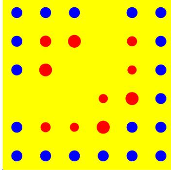
Figure 3: Optimized  $90^\circ$  waveguide bend in a 2D photonic crystal of dielectric rods. The radii of ten rods (shown in red) are modified.
