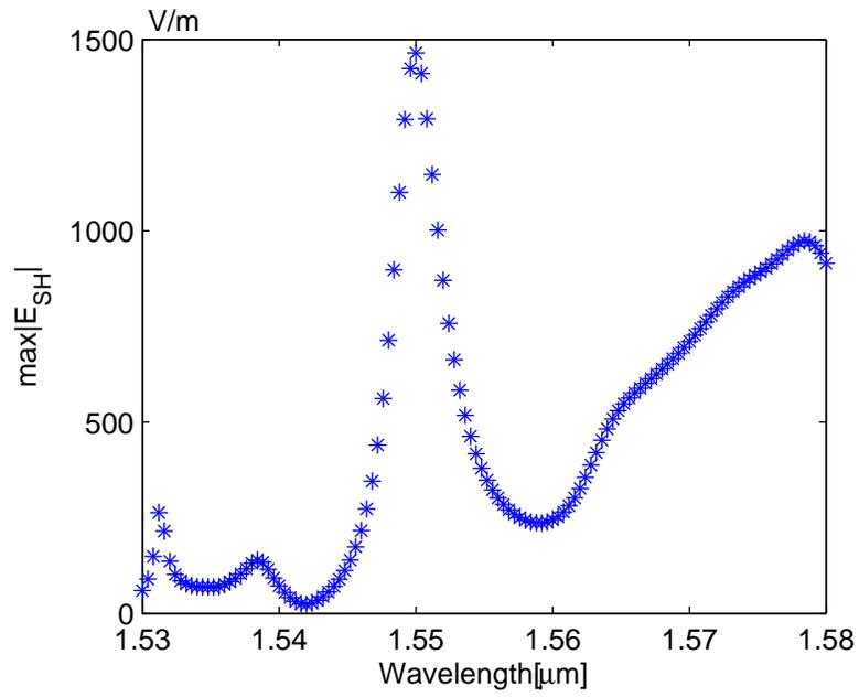
Fig. 7. The maximum amplitude of the generated second harmonic wave at  $z = a$  versus the free space wavelength of the fundamental frequency, for Example 2
