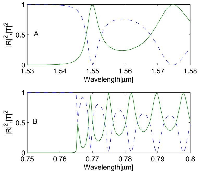
Fig. 6. Linear transmission and reflection properties of the piecewise uniform structure in Example 2. The solid and dashed lines represent  $|T|^2$  and  $|R|^2$ , respectively.
