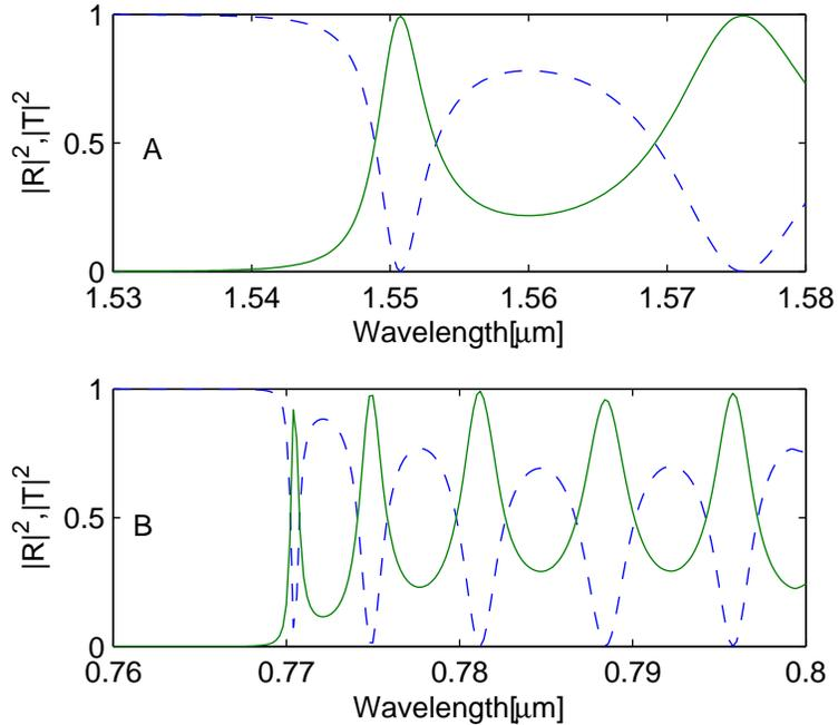
Fig. 1. Linear transmission and reflection properties of a piecewise uniform waveguide (Example 1) for two wavelength intervals. The solid and dashed lines represent  $|T|^2$  and  $|R|^2$ , respectively.
