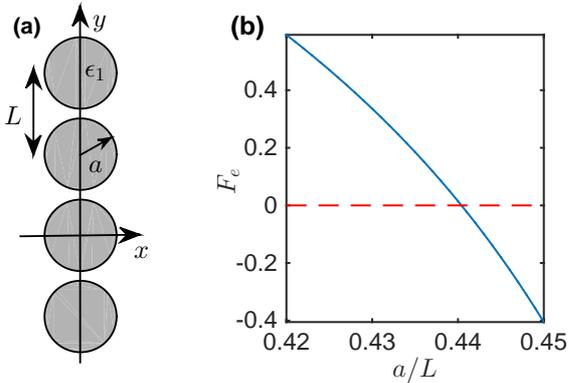
FIG. 1: (a): A periodic array of circular cylinders surrounded by air. (b)  $F_e$  (with unit  $L$ ) of the first ASW as a function of radius  $a$  for  $\epsilon_1 = 8.2$ .
