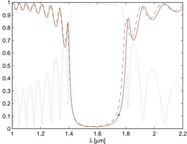
Figure 5: Transmission and reflection spectra of a metal-insulator-metal waveguide Bragg grating with  $N = 14$  periods. The dashed line is the magnitude of the scaled transmission coefficient (i.e.,  $|T_s|$ ) of Han *et al.* [32]. The solid and dash-dot lines are the magnitudes of the scaled transmission and reflection coefficients (i.e.  $|T_s|$  and  $|R|$ ) calculated by the DtN map method. For  $\lambda = 1.75 \mu\text{m}$ , a more accurate solution is shown as the little circle.
