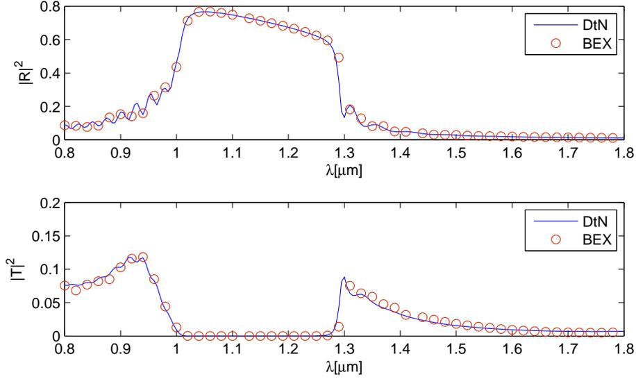
Figure 1: Reflectance and transmittance of the fundamental TM mode for a deeply etched optical waveguide grating with 20 periods. The solid lines and the small circles are the results of the DtN map method and the eigenmode expansion method based on Fourier sine series [7].
