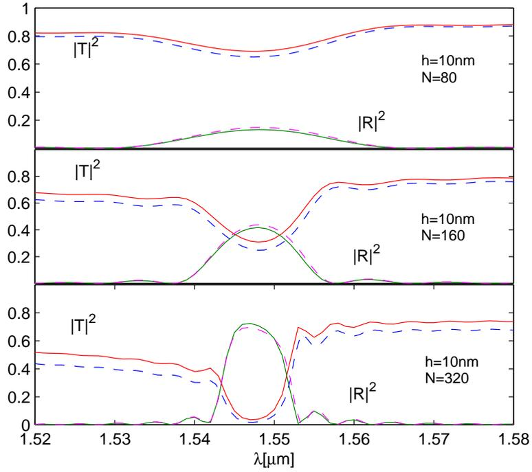
Figure 3: Reflectance  $|R|^2$  and transmittance  $|T|^2$  for a surface plasmon polariton Bragg grating with a 15 nm gold film and  $N$  symmetric gold ridges of height  $h = 10$  nm. The solid and dashed lines correspond to the DtN map method and the integral equation method [31], respectively.
