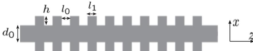
Figure 2: Schematic view of a long range SPP waveguide Bragg grating structure.
