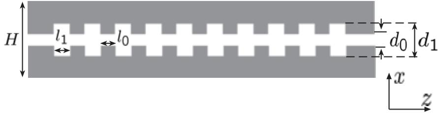
Figure 4: Schematic view of a metal-insulator-metal SPP Bragg grating structure.
