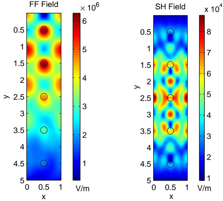
Fig. 6. Magnitudes of the fundamental frequency wave (left) and the second harmonic wave (right) for five arrays of cylinders at  $\gamma = 0.86943$ . The incident wave has a magnitude of  $10^6$  V/m and an angle of incidence  $\theta_0 = 7.6^\circ$ .
