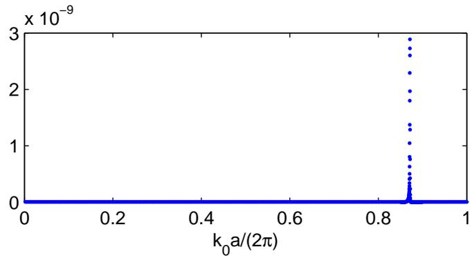
Fig. 2. Frequency dependence of the normalized reflected power of the second harmonic wave, defined in (44), for one array of cylinders. The angle of incidence the pump wave is fixed at  $\theta_0 = 8.25^\circ$ .
