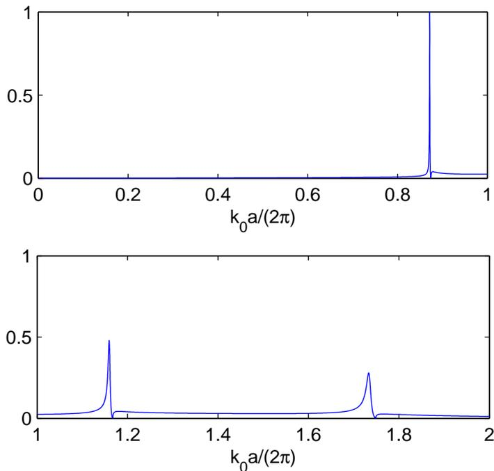
Fig. 1. Linear reflection spectrum for one array of cylinders, where the incident wave has a fixed angle of incidence  $\theta_0 = 8.25^\circ$ . The vertical axis is the power reflectivity defined in (43).
