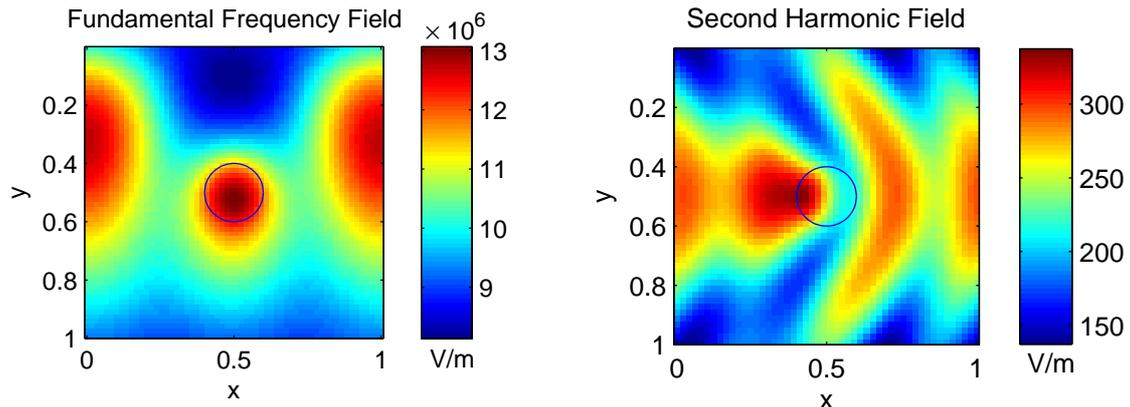
Fig. 3. Magnitudes of the fundamental frequency wave (left) and the second harmonic wave (right) for one array of cylinders at  $\gamma = 0.8714$ . The incident wave has a magnitude of  $10^6$  V/m and an angle of incidence  $\theta_0 = 8.25^\circ$ .
