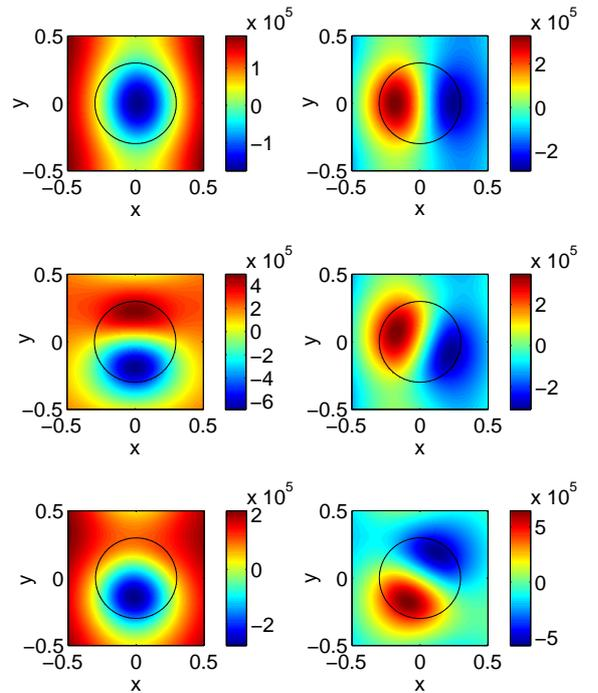
FIG. 10. Wave field patterns,  $\text{Re}(u)$  in the left and  $\text{Im}(u)$  in the right, of the three solutions marked as A, B and C in Fig. 8 (top panel), for  $A^{(i)} = \sqrt{5} \times 10^5 \text{ V/m}$  and  $\omega L/(2\pi c) = 0.53$ .
