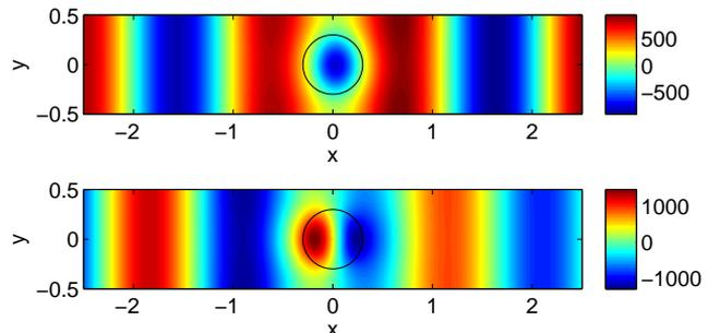
FIG. 4. Real (top) and imaginary (bottom) parts of  $u$  for the symmetric solution of the nonlinear diffraction problem at  $\omega L/(2\pi c) = 0.53$  and  $A^{(i)} = 10^3 \text{ V/m}$ .
