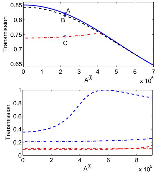
FIG. 8. Dependence of transmission coefficients on incident amplitude  $A^{(i)}$  for solutions of the nonlinear diffraction problem at  $\omega L/(2\pi c) = 0.53$ . Top panel: the symmetric and two asymmetric solutions coupled to the first NSW are shown as the solid, dashed and dash-dot lines, respectively. Bottom panel: asymmetric solutions coupled to the second and third NSWs are shown as the blue and red curves, respectively.
