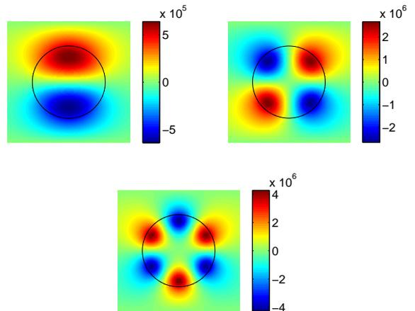
FIG. 3. Electric field patterns of the nonlinear standing waves at frequency  $\omega L/(2\pi c) = 0.53$  corresponding to points A, B and C in Fig. 2 .
