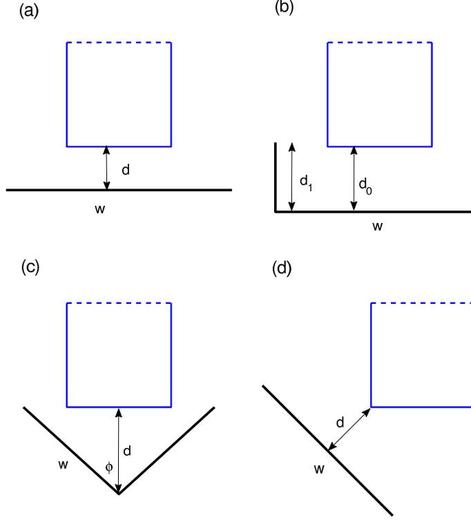
Fig. 3. For a boundary unit cell, sources are located on a horizontal line (a), a  $U$ -curve (b), or a  $V$ -curve (c). For a corner unit cell, sources are located on a line (d). Geometric parameters are: (a)  $d = 1.3a$ ,  $w = 4.8a$ ; (b)  $d_0 = 1.6a$ ,  $d_1 = a$ ,  $w = 2.25a$ ; (c)  $d = 1.28a$ ,  $w = 1.8a$ ,  $\phi = 84^\circ$ ; (d)  $d = 2a$ ,  $w = 2a$ .
