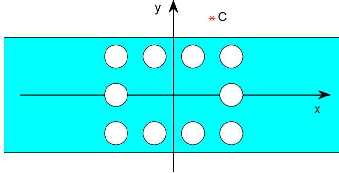
Fig. 4. A dielectric slab with ten holes forming a rectangular loop.
