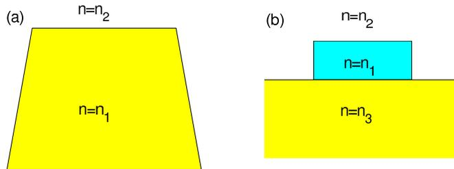
Figure 1: Optical waveguides with a waveguide core surrounded by a homogeneous medium (a) or a layered medium (b).
