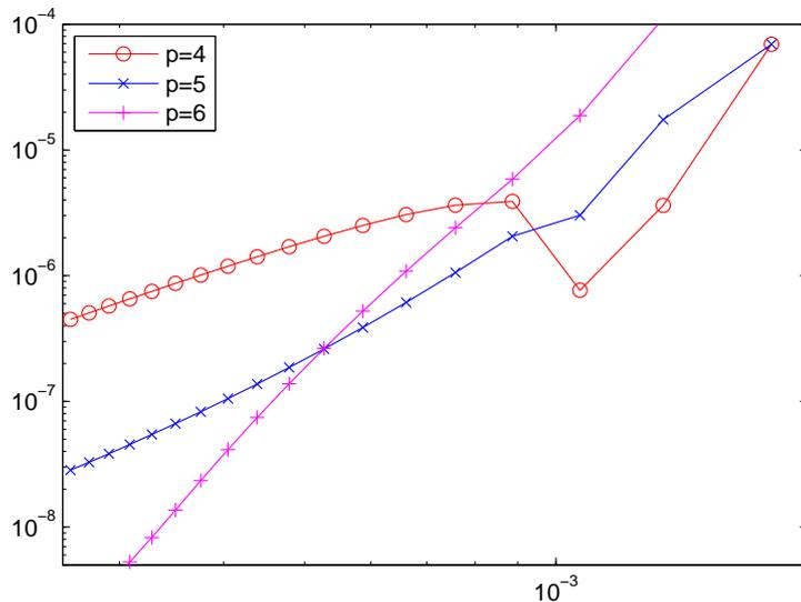
Figure 8: Dependence of the absolute error on the inverse of the matrix size of  $F$  for the rectangular waveguide with a layered background shown in Fig. 1(b).
