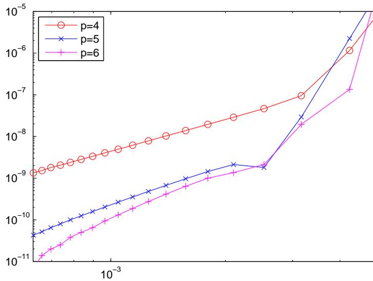
Figure 7: Dependence of the absolute error on the inverse of the matrix size of  $F$  for the drop-shaped waveguide shown in Fig. 2(c).
