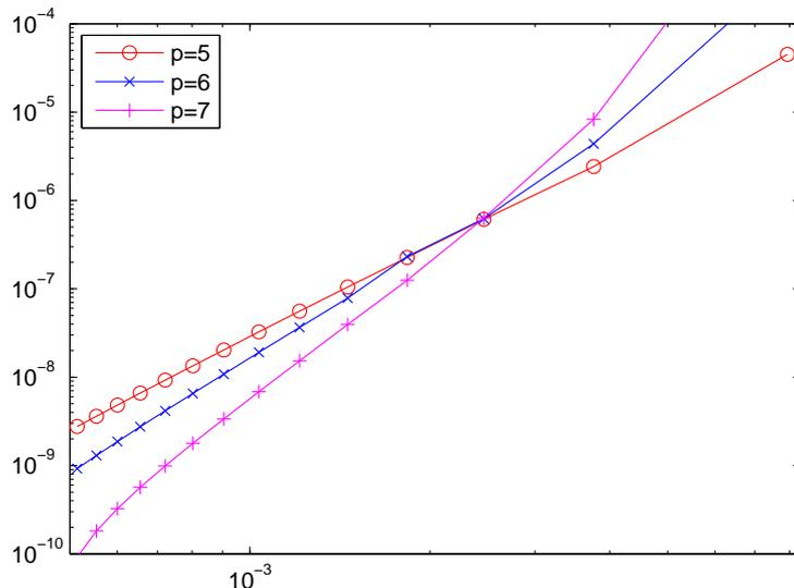
Figure 4: Dependence of the absolute error on the inverse of the matrix size of  $F$  for the bounded waveguide shown in Fig. 2(a) and  $n_1 = \sqrt{8}$ .
