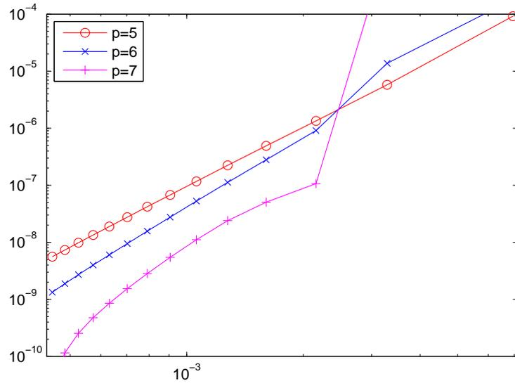
Figure 5: Dependence of the absolute error on the inverse of the matrix size of  $F$  for the square waveguide shown in Fig. 2(b).
