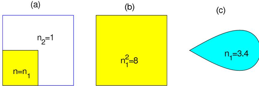
Figure 2: (a) A bounded waveguide, (b) an open square waveguide, (c) an open waveguide with a drop-shaped core.
