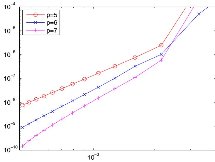
Figure 6: Dependence of the absolute error on the inverse of the matrix size of  $F$  for the trapezoidal waveguide shown in Fig. 1(a).
