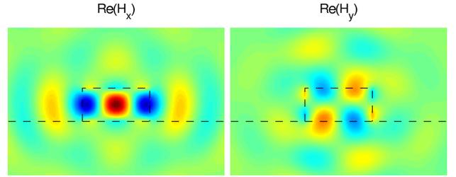
Fig. 3. Transverse magnetic field patterns of a complex mode for waveguide (b) in Fig. 1.
