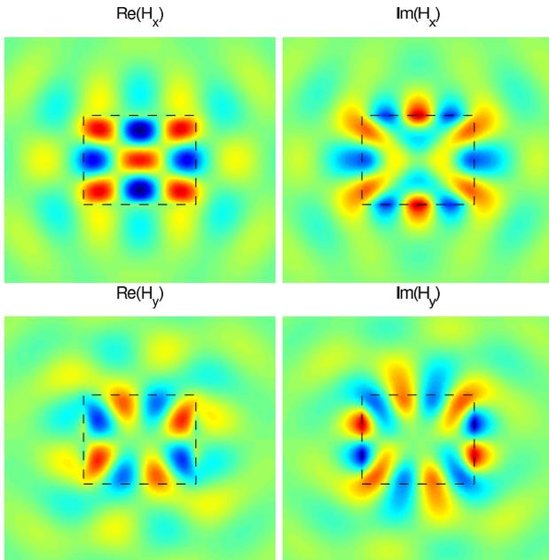
Fig. 2. Transverse magnetic field patterns of a complex mode for a waveguide (a) in Fig. 1.
