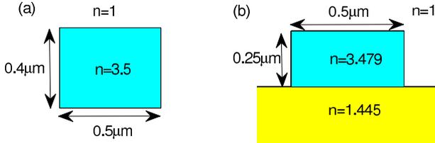
Fig. 1. Two open waveguides.
