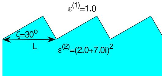
Fig. 4. A metallic echelette diffraction grating.
