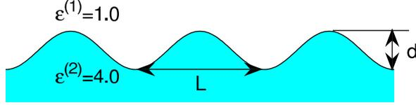
Fig. 2. A dielectric sinusoidal diffraction grating.
