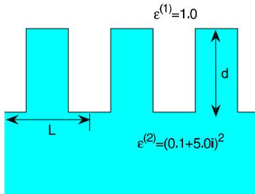
Fig. 3. A metallic lamellar diffraction grating.
