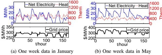
Fig. 4: Net electricity demand and heat demand for a typical week in January and May. The net demand is computed by subtracting the wind generation from the electricity demand.
