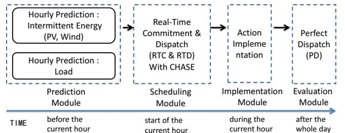
Fig. 1: Proposed implementation of CHASE in microgrids
