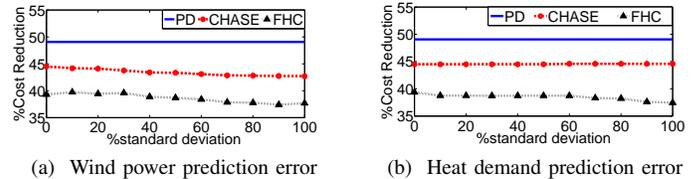
Fig. 7: Cost reduction as a function of the size prediction error.
