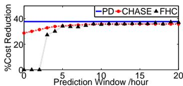
Fig. 6: Cost reduction as a function of perfect prediction window length.
