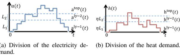
Fig. 2: The demand division sub-process. CHASE always deliver the demand to the generator with large capacity.
