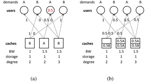
Fig. 3: A simple example demonstrating the usefulness of fractional storage. The system has the same setup as that in Figure 1. In (a), the videos are stored in full. Even with the optimal topology, the oracle server still needs to fill in the gap of half of a video. In (b), with fractional storage and streams, caches can fully serve users even with less storage.
