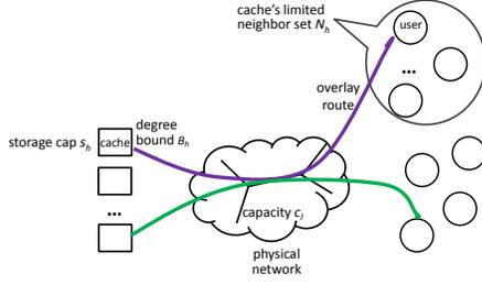
Fig. 2: Caches and users connected by a physical network. The link capacity constraints can exist arbitrarily anywhere in the network.
