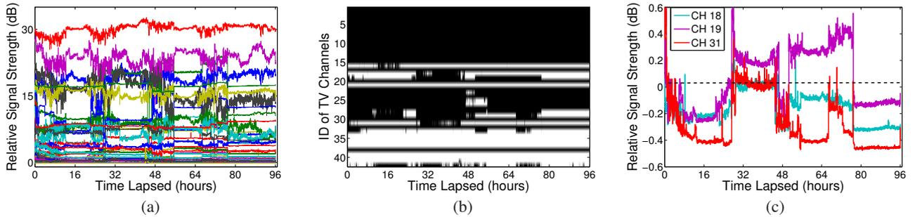
Figure 3: (a) Relative signal strength (in dB) for all 42 TV channels in a 96-hour window. (b) Channel occupancy statuses for all 42 channels in the same 96-hour window. White spaces are denoted in white, and occupied channels in black. (c) Three TV channels (CH 18, 19 and 30) that move up and down around the white space thresholds (e.g., the dotted line). They become white spaces from time to time.
