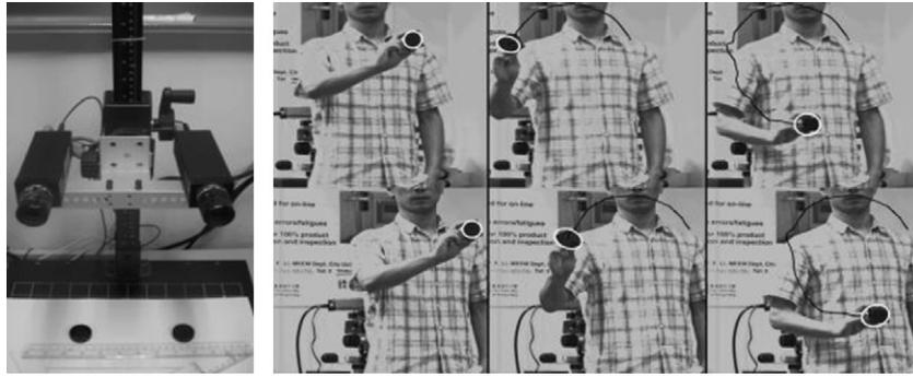
Fig. 9. Vision system setup and snapshots of the stereo trajectory tracking.
