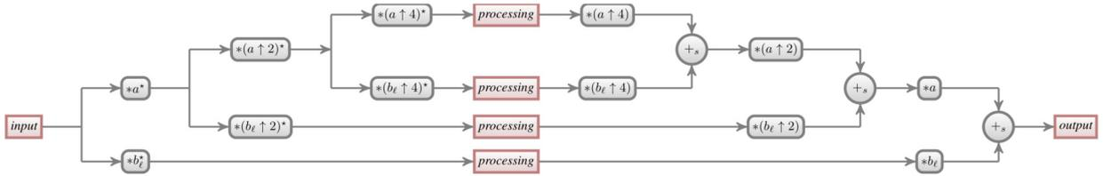
**Fig. 5.** Undecimated discrete framelet transforms (UDFmT) associated with a filter bank  $\{a; b_1, \dots, b_s\}$ . Each box with  $b_\ell$  runs through  $\ell = 1, \dots, s$  and the circle with  $+_s$  sums over all  $s$  outputs from boxes with  $b_\ell$ .
