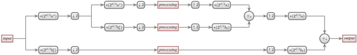
Fig. 4. Multi-level discrete framelet transforms (DFmT) associated with a filter bank  $\{a; b_1, \dots, b_s\}$ . Each box with  $b_\ell$  runs through  $\iota = 1, \dots, s$  and the circle with  $+_s$  sums over all  $s$  outputs from boxes with  $b_\ell$ .
