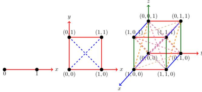
Fig. 7. Left to Right: Directional Haar tight framelet filter banks in  $d = 1, 2, 3$  respectively, where each line connecting two vertices  $\gamma_1, \gamma_2 \in \{0, 1\}^d$  represents a high-pass filter  $b := 2^{-d}(\delta_{\gamma_1} - \delta_{\gamma_2})$ .
