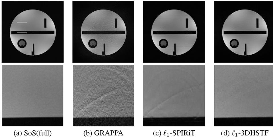
**Fig. 12.** Reconstruction results on 32% K-space data by the uniform sampling mode (one line taken from every four lines) with 48 ACS lines in Fig. 10(b). (a) SoS image of the full K-space with zoom-in part; (b) GRAPPA [16]; (c)  $\ell_1$ -SPIRiT method [34] with parameter 0.005; (d) the  $\ell_1$ -3DHSTF method with parameter 0.003. The second row is the zoom-in parts of first row, respectively.
