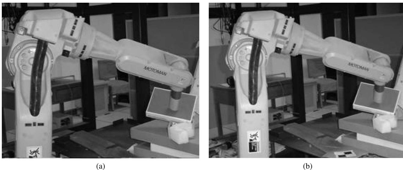
Fig. 9. Scenes of experiments in the end stage. (a) Scene with pose-based method and (b) scene with position-based method.
